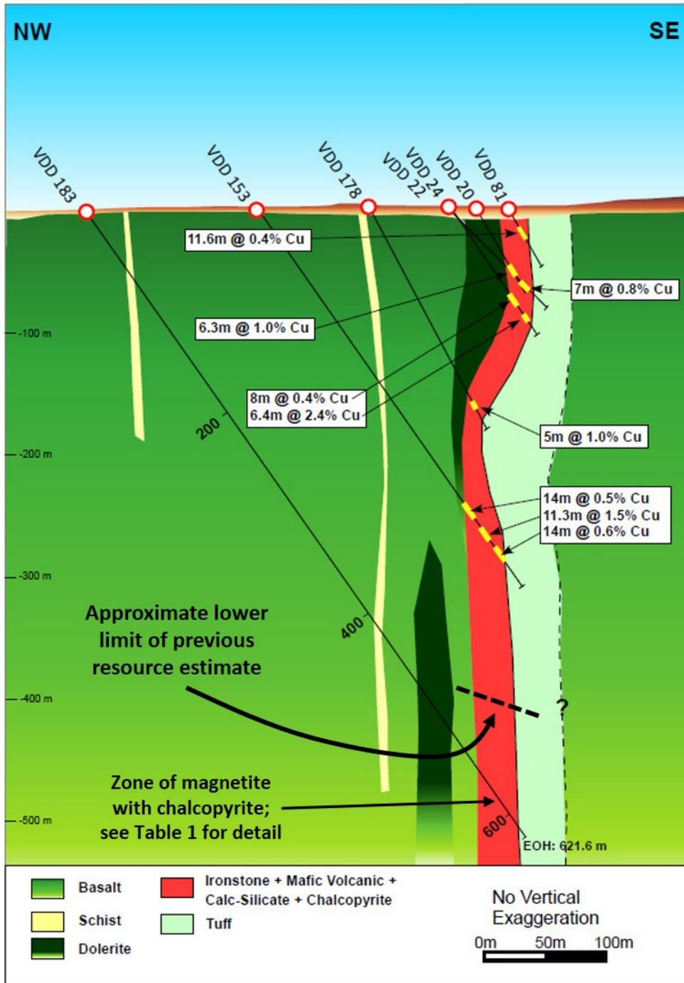
Figure 3: Drill hole cross section containing VDD 183 and previously drilled diamond holes
