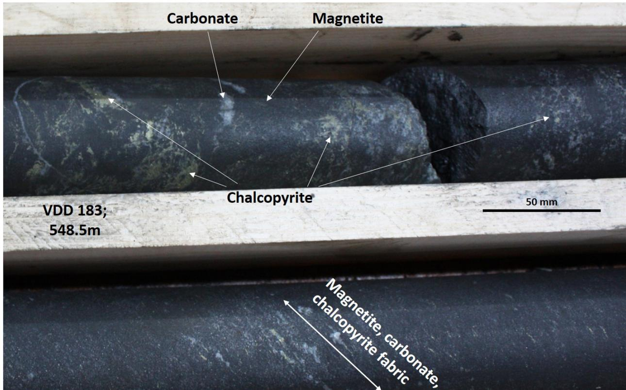
**Figure 2: drill core from VDD 183 at 548.5m showing blebby chalcopyrite, and magnetite-chalcopyrite-carbonate foliation**
